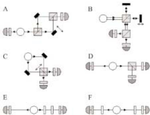
Figure 4. Six experiments with single photons that can be used for understanding quantum mechanics. The circles represent the source of photon pairs, the squares with a diagonal line are beam splitters, the dark rectangles are mirrors, the light rectangles are either energy filters or polarizers, and the half-circle symbols represent the photon detectors.
