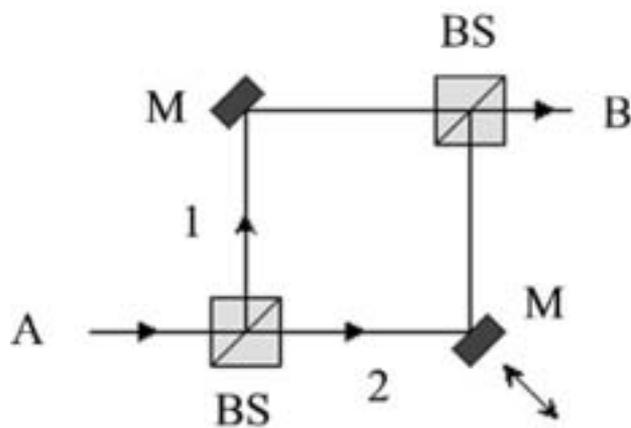
Figure 1. The Mach-Zehnder interferometer has two beam splitters (BS) and two mirrors (M). A photon going from A to B can take either path 1 or 2.
