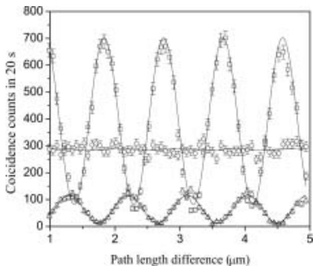
Figure 3. Data for the experiment on the quantum eraser as a function of the difference in length between the two arms of the interferometer. The solid lines are fits to the data.
