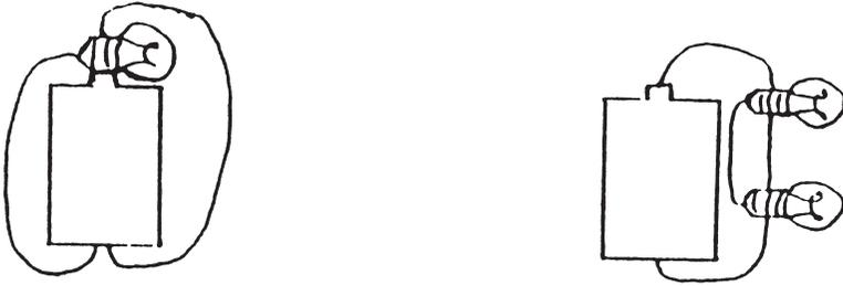
Some students were able to identify series and parallel circuits when two batteries were touching each other but not when the batteries were connected by wires. Additional activities setting up circuits with batteries, bulbs, and wires, making and checking predictions, and recording and discussing results helped students on later evaluations to identify series and parallel circuits when the batteries were not directly touching. (See Figure 4.)
